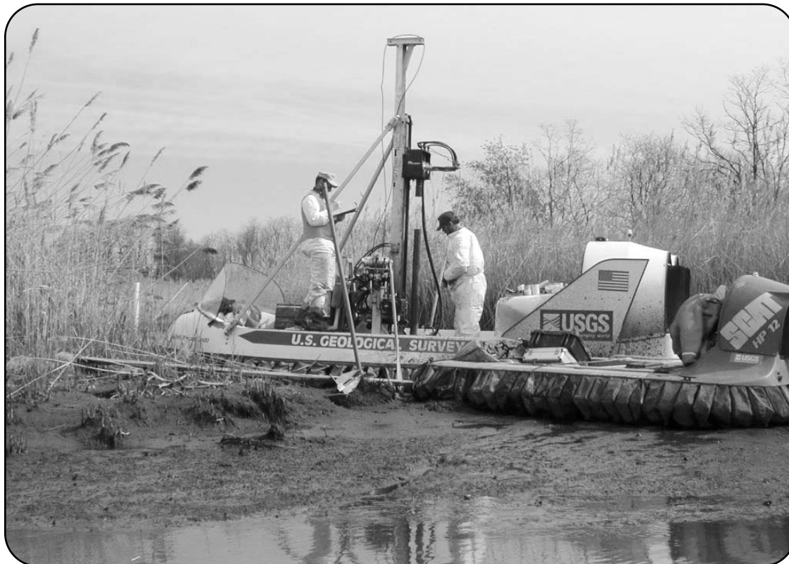
The Hoverprobe 2000 co-developed by the USGS with industry partners to drill in wetland areas. The skirt at the base of the craft traps pressurized air, allowing the craft to fly over land, water, ice, snow, or mud. The drill rig can cut a hole and collect core samples to a depth of about 100 feet or it can install a monitoring well rapidly. No fluids are used or injected into the ground.
