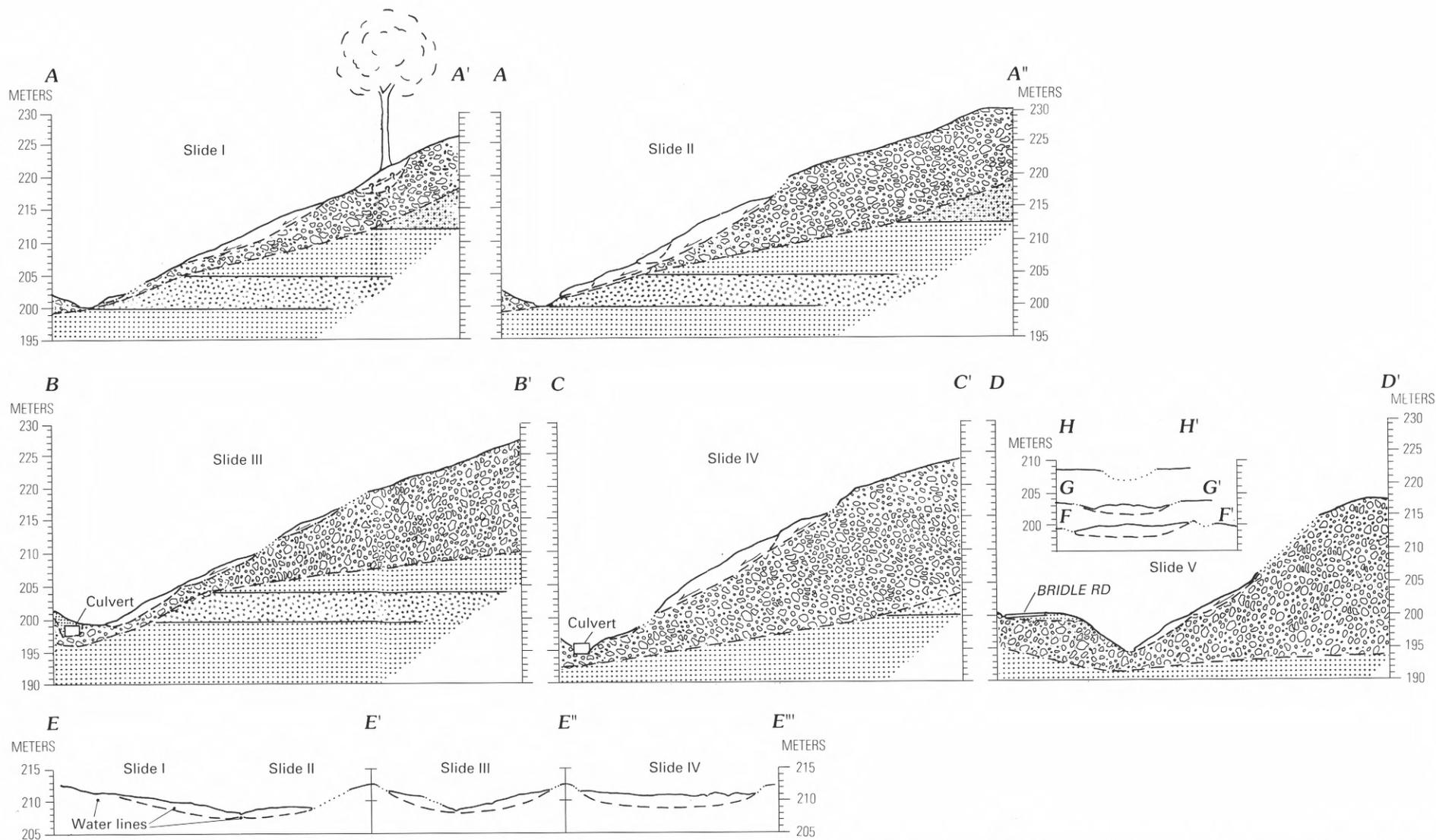
**Figure 8.** Plane-table map of the Bridle Road landslide complex (thin landslides in till) by C. Scott Brockman, University of Cincinnati, March 1982 (modified from Brockman, 1983, pl. 5). Base datum established from Hamilton County topographic map of the Dry Run Creek area, Anderson Township. Contour interval 1 meter.
