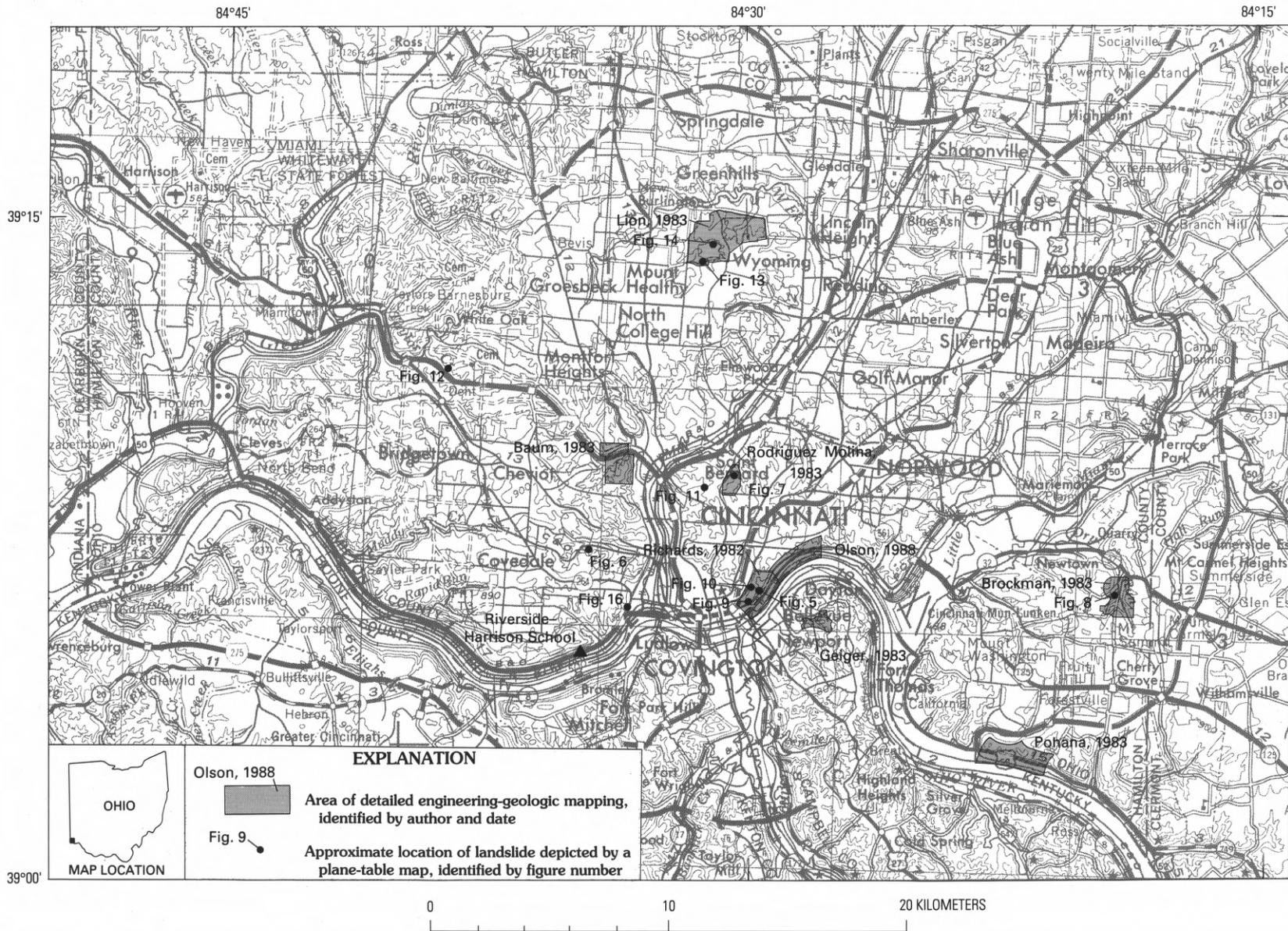
**Figure 1.** Map of Cincinnati and Hamilton County, Ohio, showing approximate outlines of areas of detailed engineering-geologic mapping by students at the University of Cincinnati and locations of landslides depicted by plane table maps. Base from U.S. Geological Survey 1:250,000 Cincinnati, Ohio; Indiana; Kentucky (1953, revised 1974). Contour interval 100 feet.
