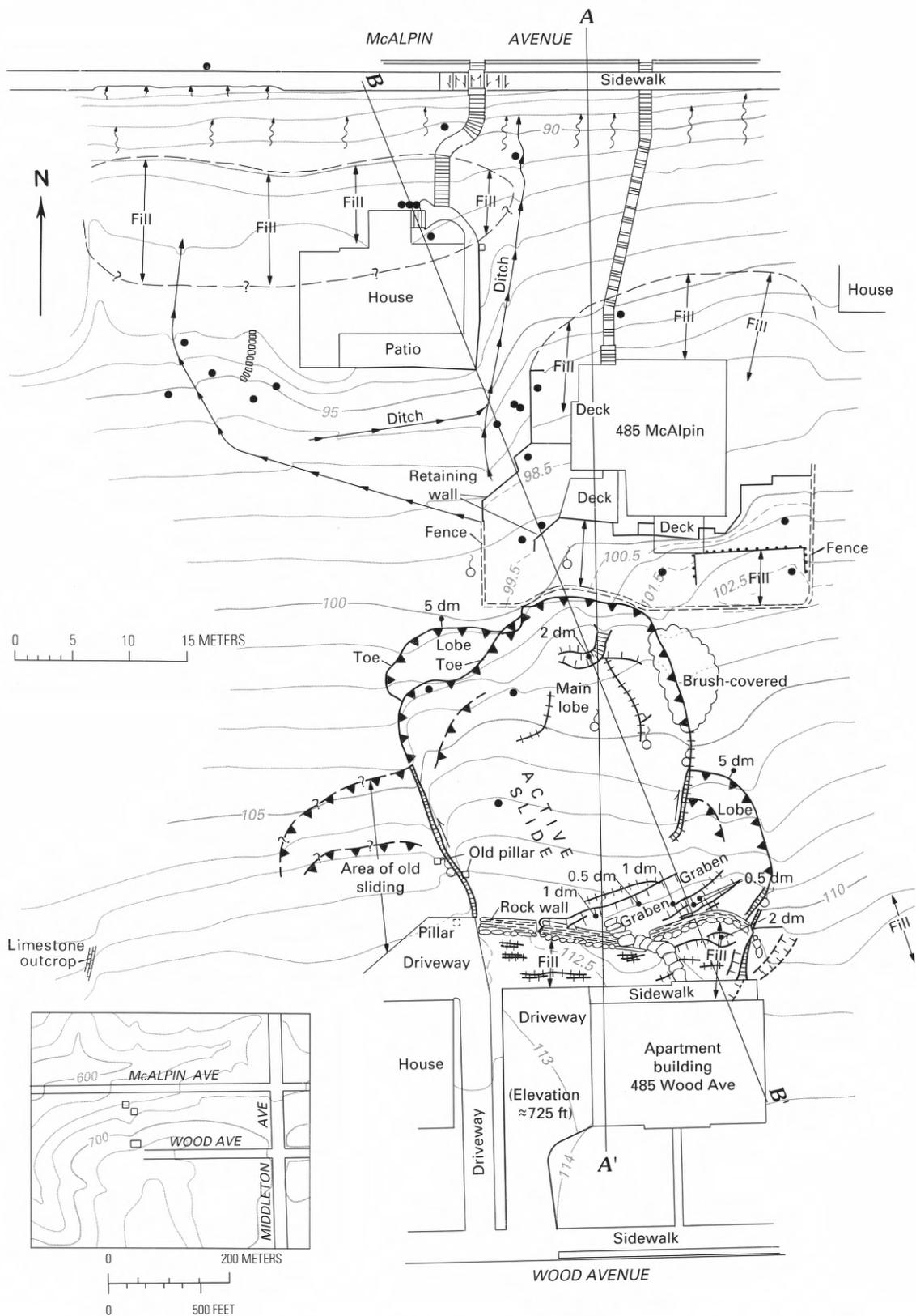
**Figure 11 (above and facing page).** Plane-table map of a landslide between Wood Avenue and McAlpin Avenue, by Arvid Johnson, University of Cincinnati, April 1980. Contour interval 1 meter (arbitrary datum); intermediate contours dashed; approximate contours dotted. Dashed outline for fill, queried where extent uncertain. Buildings, steps, rock wall, and sidewalks are schematic. Inset map contour interval 25 feet (datum is mean sea level).
