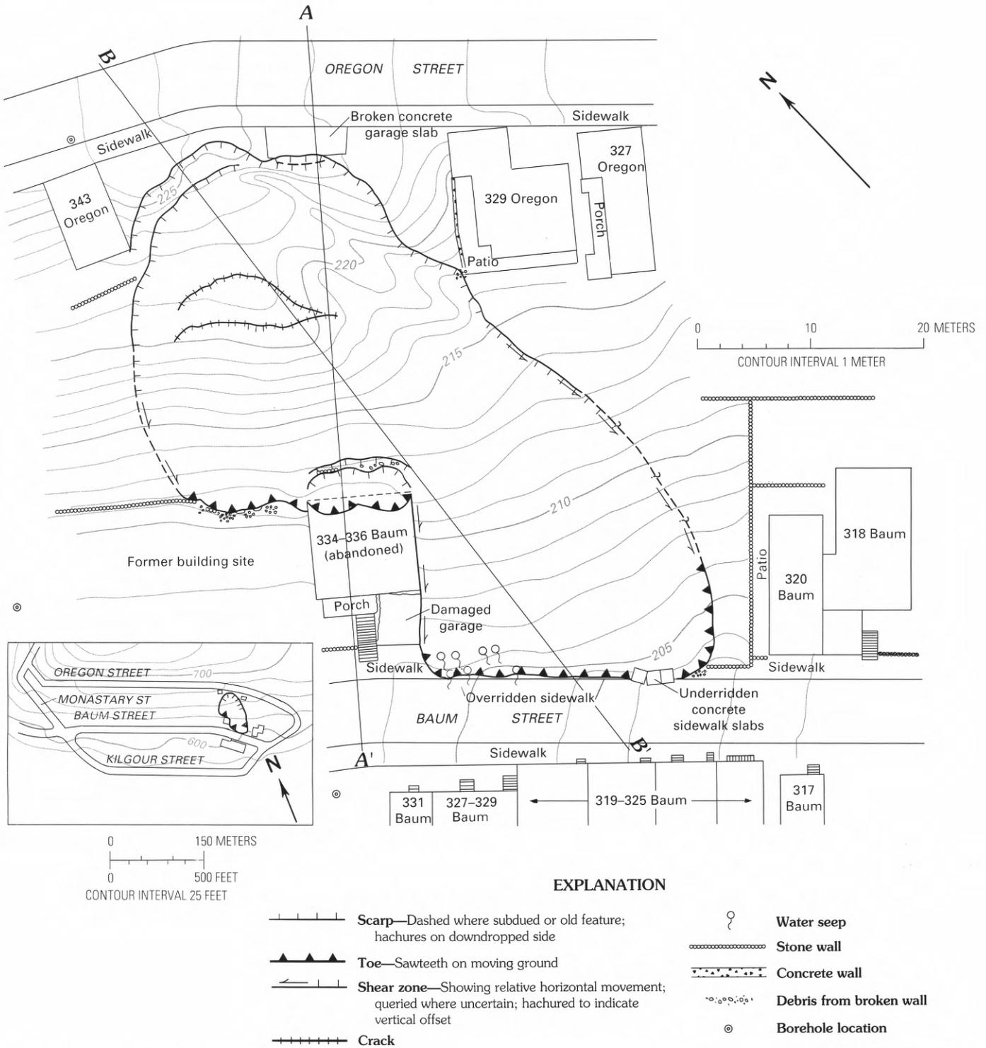
**Figure 9 (above and facing page).** Plane-table map of the Oregon Street and Baum Street landslide in Mount Adams, by N.B. Patterson and K.A. Richards, University of Cincinnati, spring 1981 (modified from Richards, 1982, pl. 3). Map contours defined by arbitrary datum on Baum Street; index map datum is mean sea level. Buildings, steps, sidewalks, and walls are schematic.
