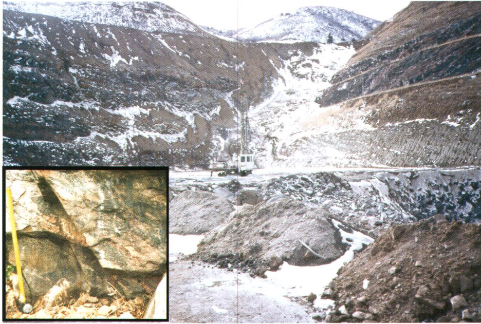
Figure 6. Specification Aggregate Quarry (Lafarge Corporation) near Golden, Colo., mines Precambrian banded gneiss for making crushed stone. Highwalls and benches indicate volume of material already mined. Drill rig (center) is preparing holes for blasting charges. Inset shows closeup of pink and black banded gneiss crushed at quarry.
