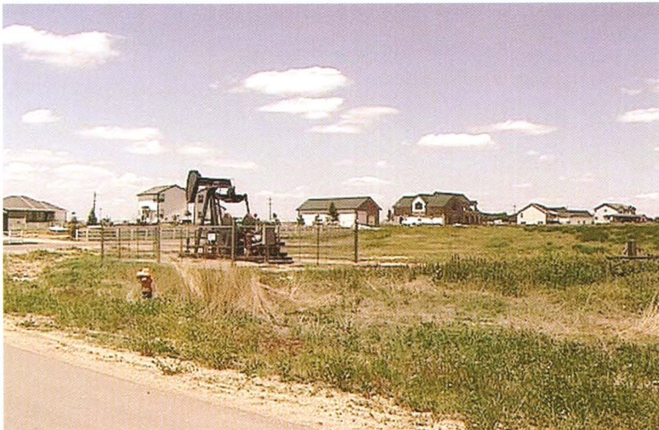
Figure 18. An established oil well pump jack in an actively developing residential area. Regulations limit how close new housing can be built to the pump jack. Even though this well might be purchased, plugged, and abandoned, developers still must design around the well for safety reasons.
