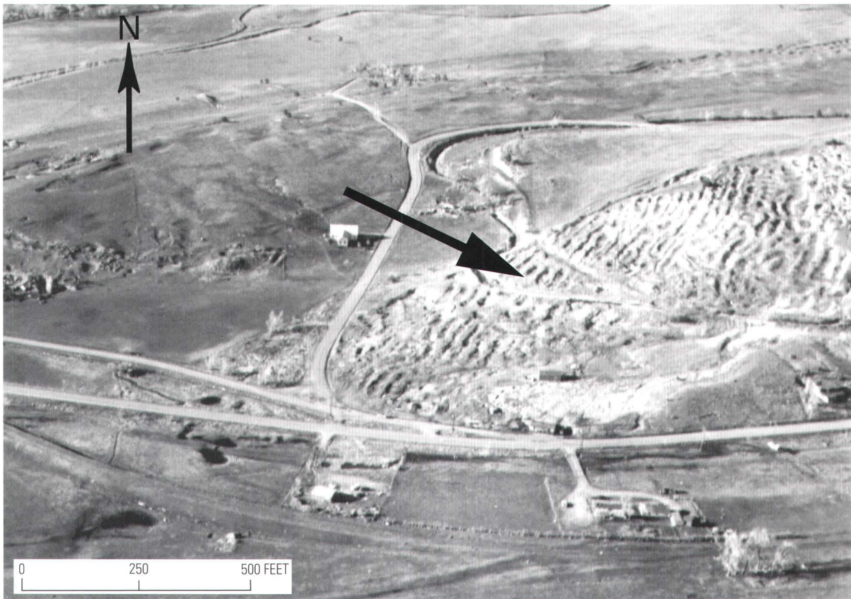
Figure 12. Aerial photograph of ground over coal mine subsidence (arrow). Photograph was taken near southwestern part of Boulder-Weld coal field (fig. 9) south of Boulder, Colo. Morphology of subsided area reflects room (lows) and pillar (ridges) mining method used to extract coal.
