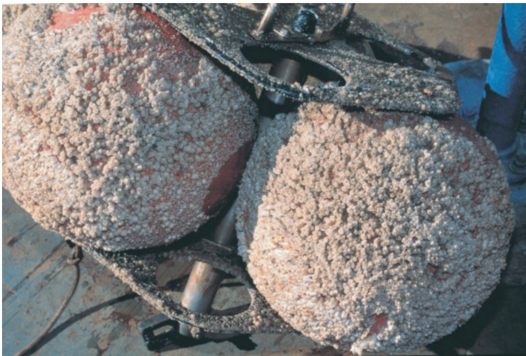
Figure 27. (A) Surface of a 41-inch subsurface float that was deployed at about 10 meters and (B) tripod recovery floats that were deployed about 3 meters above the bottom from September 1998 to February 1999. Both floats were deployed without anti-fouling paint. Extensive barnacles grew on the lower floats during this period, while only a thin layer of organic material grew on the upper float. The color of both floats when deployed was orange. Photographs by Dann Blackwood, U.S. Geological Survey.
