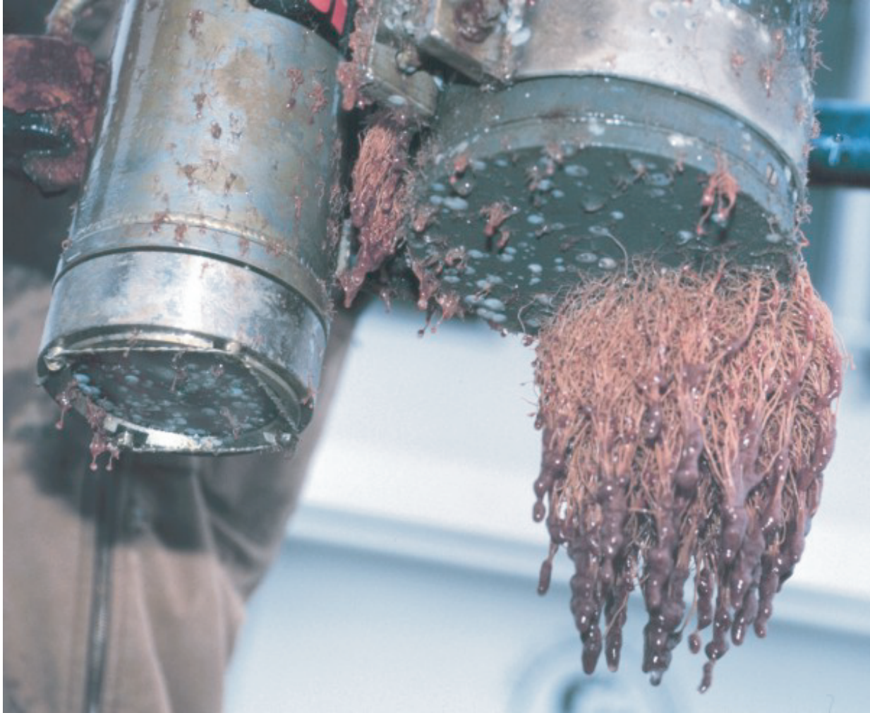
Figure 29. The lens of the bottom camera (left) and battery case (right) deployed from May to September 1999 on mooring 569 at site LT-A. Photograph by Dann Blackwood, U.S. Geological Survey.
