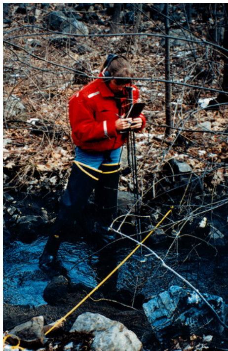
Figure 7. Cambridge Water Department staff member measuring streamflow in an ungaged tributary to Stony Brook Reservoir near Weston, Massachusetts.
