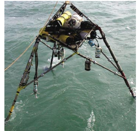
Figure 2. Photograph of USGS tripod designed to measure currents and sediment transport being deployed at the 10-m Chienti River site.
