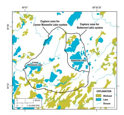
**Figure 4.** Model simulated ground-water capture zones for two lakes demonstrate that lakes receive water from distant areas as well as nearshore areas. A lake's capture zone also includes areas that contribute water to the streams that flow into a lake. Given sufficient time, lakes are affected by land-use change that occurs anywhere within their capture zone (modified from Graczyk and others, 2003).
