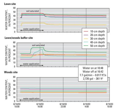
**Figure 5.** Soil-moisture profiles for the Walworth County site for a water-addition experiment along a transect that included an upslope lawn site, an intermediary buffer site, and a downslope wood site (Graczyk and Greb, 2006).
