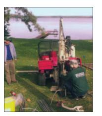
Wells were installed for ground-water sampling using a soil probe mounted on a four-wheel drive all-terrain vehicle. This allowed the wells to be installed with minimum disturbance in the lawn and wooded sites, and ensured shallow and deep ground water was included in the sampling.
