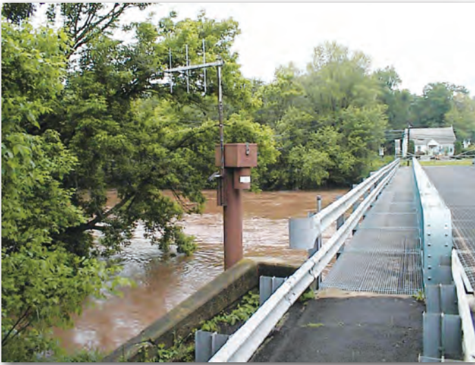
Figure 2. Flooding at U.S. Geological Survey stream gage 01398102 on the South Branch Raritan River at South Branch, New Jersey.
