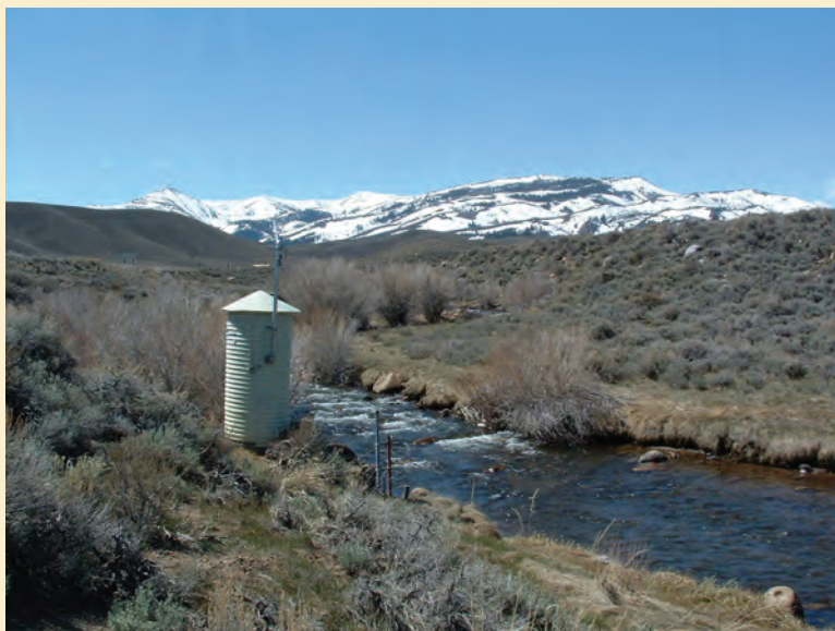
A typical U.S. Geological Survey streamgage on the Little Walker River near Bridgeport, Nevada.
