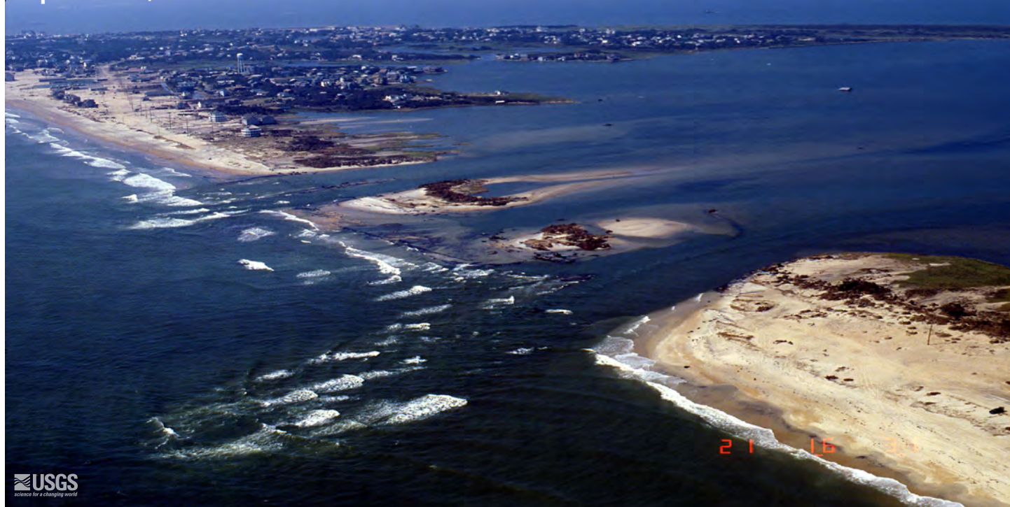
Figure 2. Hurricane Isabel opened a breach in the island southwest of Cape Hatteras. Combined waves and storm surge attacked the island where the dunes were lowest and the island was narrowest.
