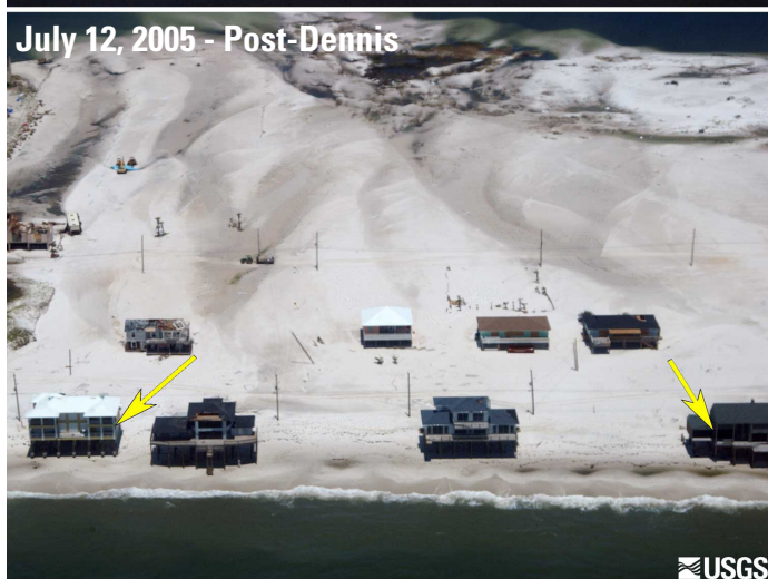
Figure 3. Navarre Beach, Florida. On this part of Navarre Beach, overwash deposits from Hurricane Dennis extend farther landward than overwash deposits from Hurricane Ivan. Deposits from both storms covered the two coast-parallel roads. (Arrows in all images point to the same features.)
