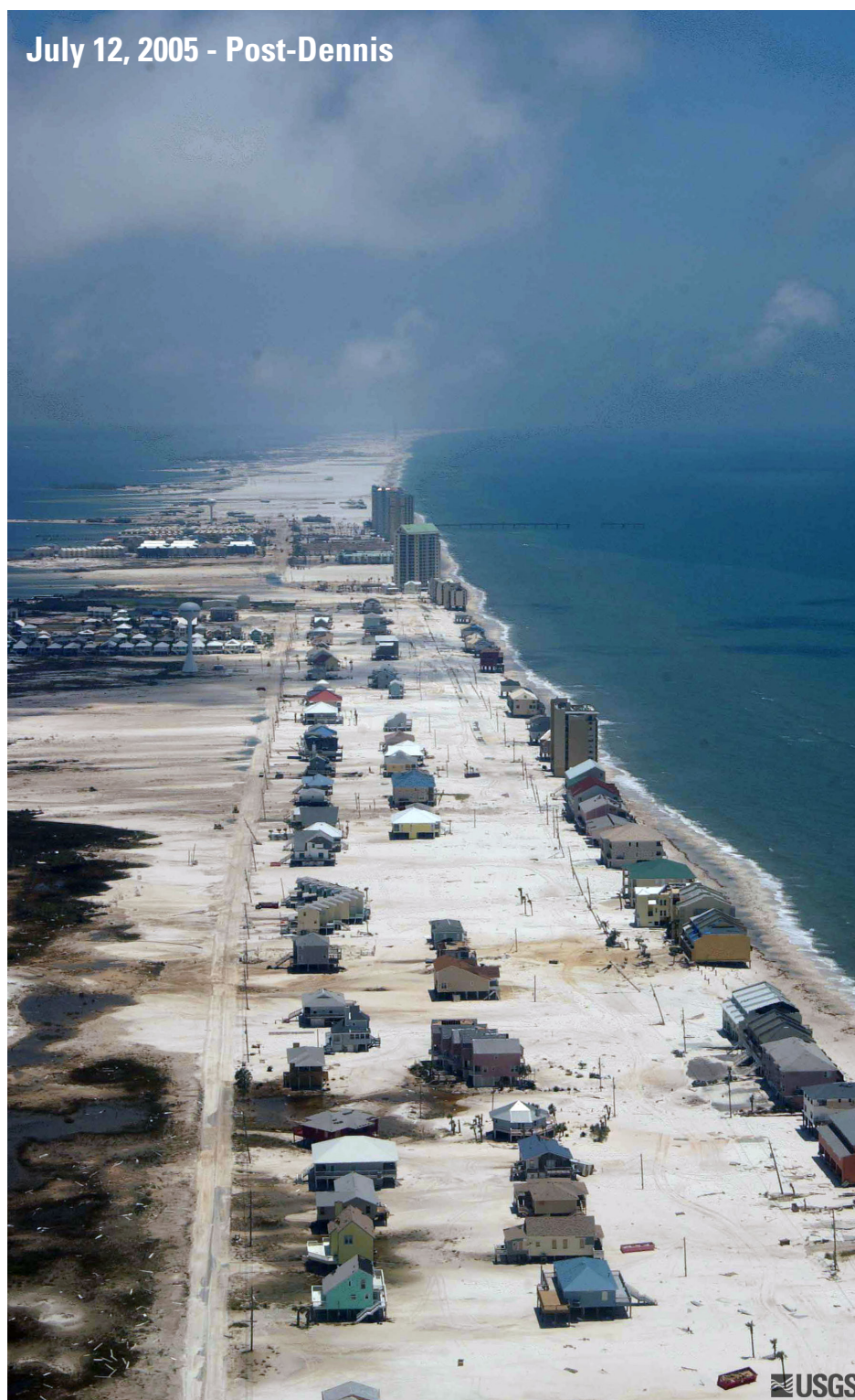
Figure 2. Santa Rosa Island, Florida, suffered severe erosion and overwash during Hurricane Dennis. Looking east, the magnitude of the overwash is evident. Overwash fans extend northward across the island, covering roads with sand eroded from the beach and dunes. In some cases, the overwash extends into the back bay.
