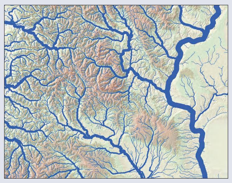
Using integrated geospatial data and hydrologic modeling to predict streamflow. Line-width is proportional to modeled streamflow.
