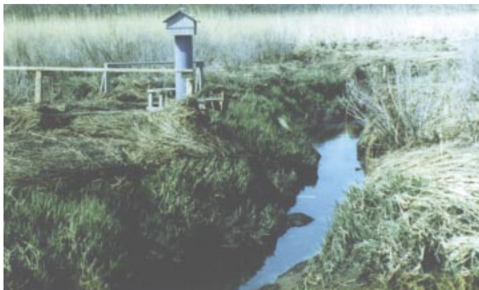
Figure 1. Automated water-level and water-quality monitoring station at Namskaket Marsh, near Orleans, Cape Cod, Massachusetts.
