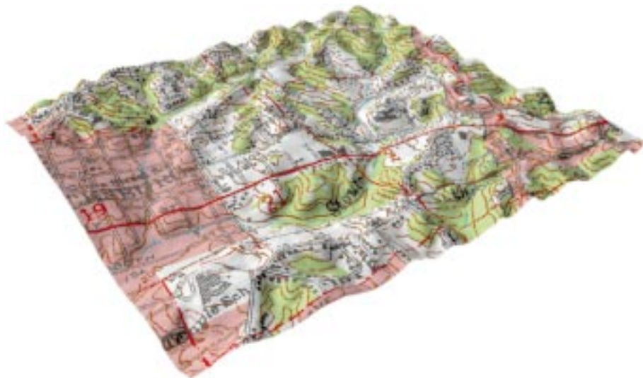
Figure 4. Aerial perspective of the terrain at Vicksburg with a topographic map superimposed upon it to aid visualization. (Created from digital raster graphic and digital elevation model data.)
