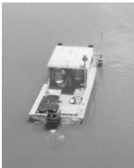
Figure 2. Using an acoustic Doppler current meter to collect three-dimensional velocity data.
