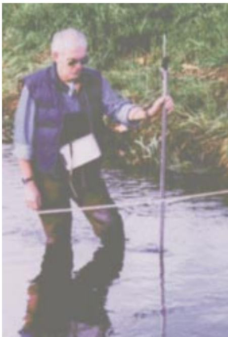
Figure 3. Measuring the flow in a Washington stream to calibrate a streamflow-gaging station.
