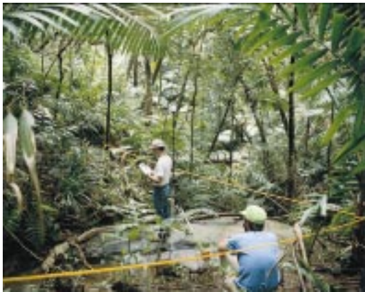
Figure 6. WEBB personnel mapping stream channels in the Luquillo Experimental Forest in northeastern Puerto Rico. Normal mapping techniques underrepresent stream networks in this tropical mountain setting due to the dense forest canopy, necessitating the use of Global Positioning System techniques to determine stream channel and headwater locations and extents.
