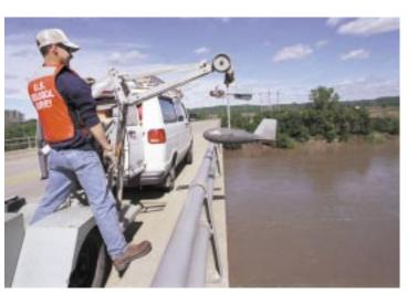
Checking the health of the Nation's rivers. Measuring flow from a bridge near a USGS streamgage.
