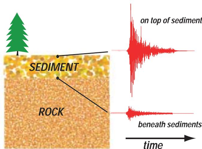
*When waves of a small earthquake impinge on the boundary between hard rock and overlying sediments from below (lower seismogram), they become amplified as they travel through the sediments to the surface (upper seismogram). A seismogram records the wave motion over time. The amplifying effects of thick sediments above the New Madrid seismic zone results in motions at the surface that are many times larger than below. (Courtesy of C. Langston, The University of Memphis.)*
