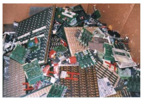
**Figure 1.** Circuit boards are sought after by recyclers for their metals content, especially gold and silver. Photograph courtesy of Melissa Goodrich, Recycling Today.
