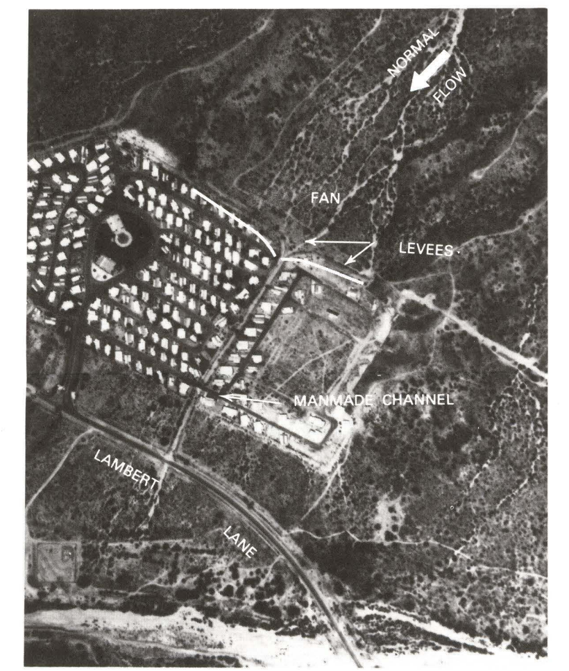
Figure 7.—Flood-proofing measures protecting a mobile home park north of Lambert Lane just east of the map area, sec. 12, T. 12 S., R. 13 E.
