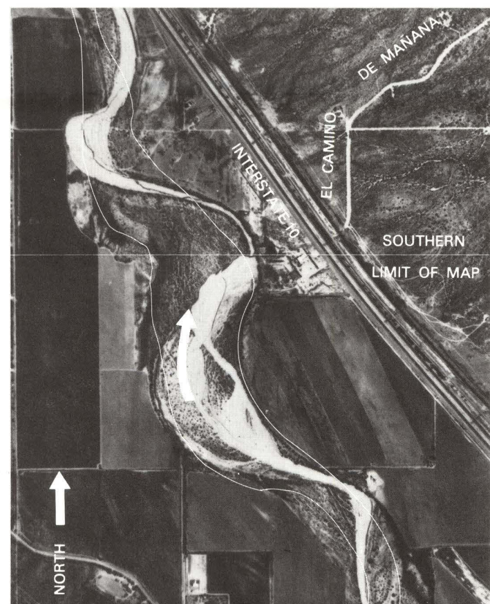
Figure 2.—Meandering channel of the Santa Cruz River near Interstate Highway 10 and El Camino De Marana in secs. 15, 16, 21, and 22, T. 12 S., R. 12 E. The white area is the low-water channel on May 5, 1966. The line is the boundary of the flood channel in February 1936. The arrow indicates the direction of flow. Scale: 1 in. = about 2,000 ft.
