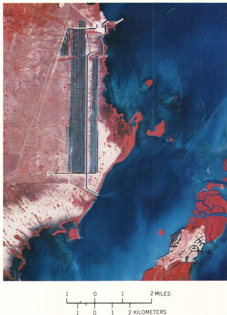
The extensive system of canals is used to cool water from the nuclear power plant at Turkey Point.
