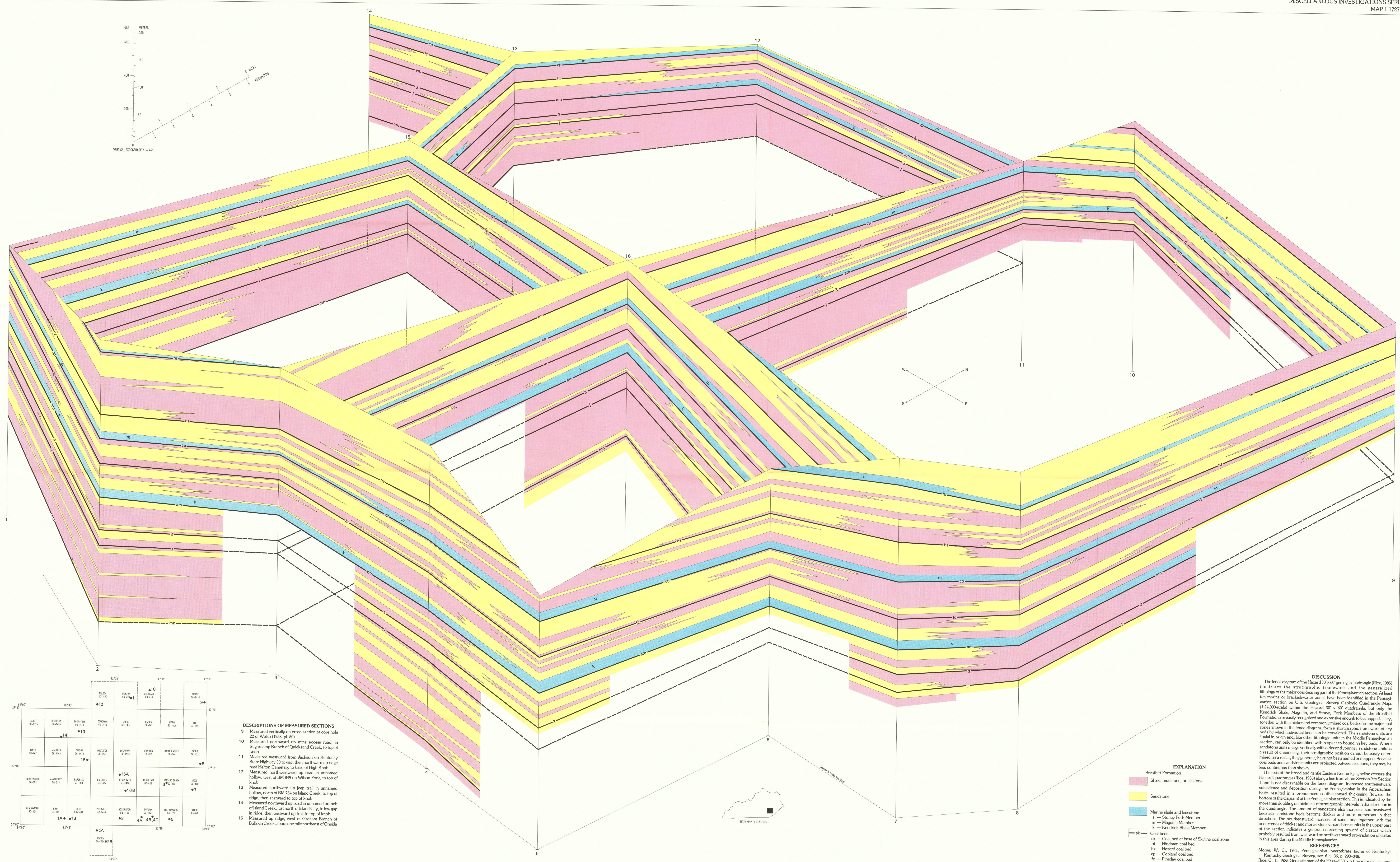
GENERALIZED FENCE DIAGRAM SHOWING PRINCIPAL COAL AND KEY MARINE BEDS OF PENNSYLVANIAN AGE IN THE HAZARD 30' x 60' QUADRANGLE, EASTERN KENTUCKY
