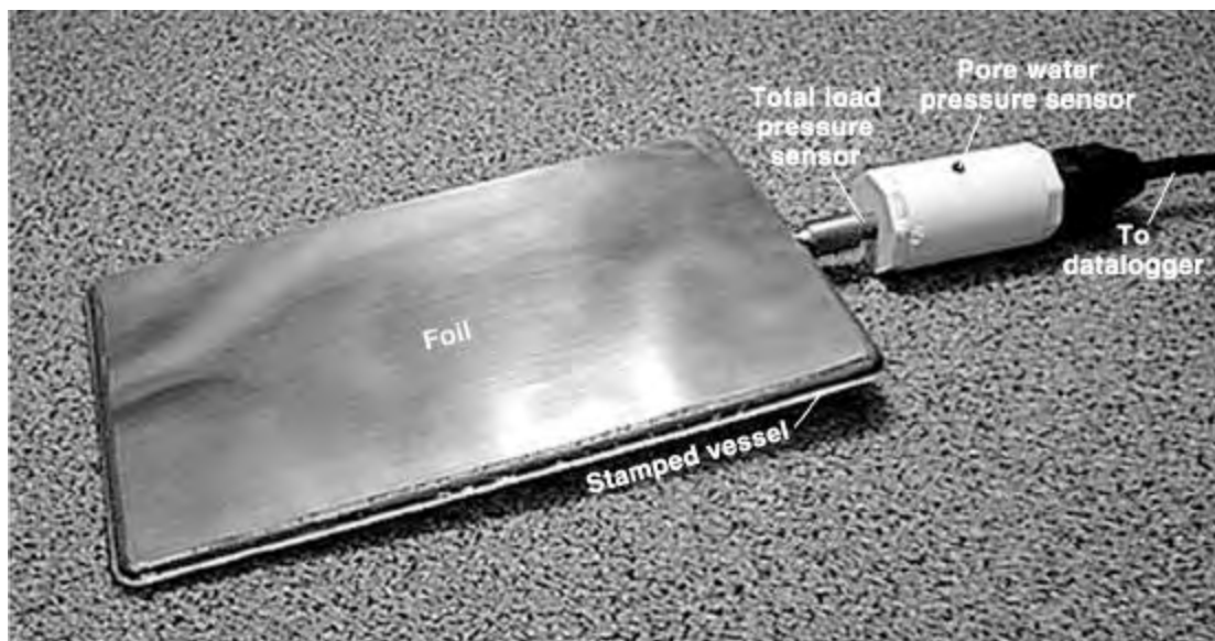
Figure 3. Load-cell scour sensor.
