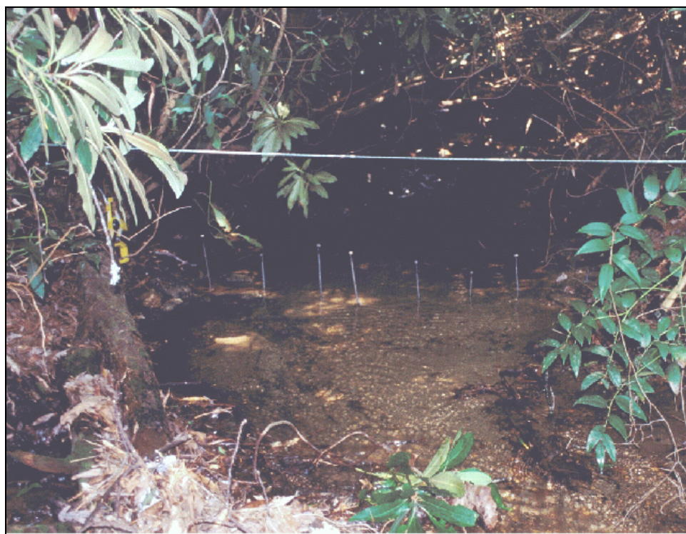
Figure 4 Example showing scour and deposition pin transect – note: pins are elevated to show locations. Actual pins were installed nearly flush with streambeds to minimize flow disturbance.
