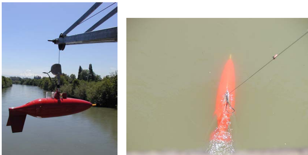
Figure 3 ( left ) The LISST-SL shown suspended from a bridge on the Puyallup river, Washington, from the B-reel frame. ( right ) View, looking down from the bridge of ‘fish in water’ shows the instrument aligned with flow, as indicated by the wake.
