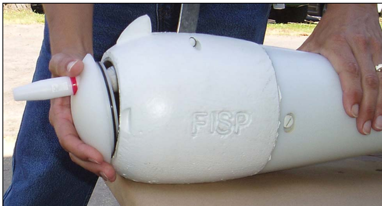
Figure 7 Insertion of nose with nozzle and bag into US DH-2.
