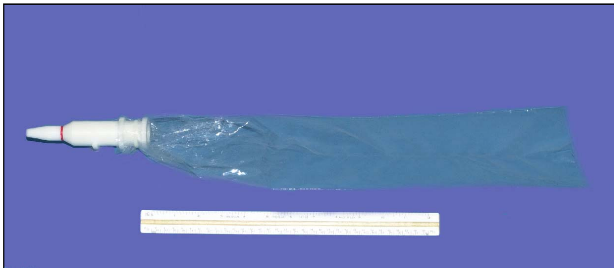
Figure 2 US D-96 nozzle holder with nozzle and bag attached.
