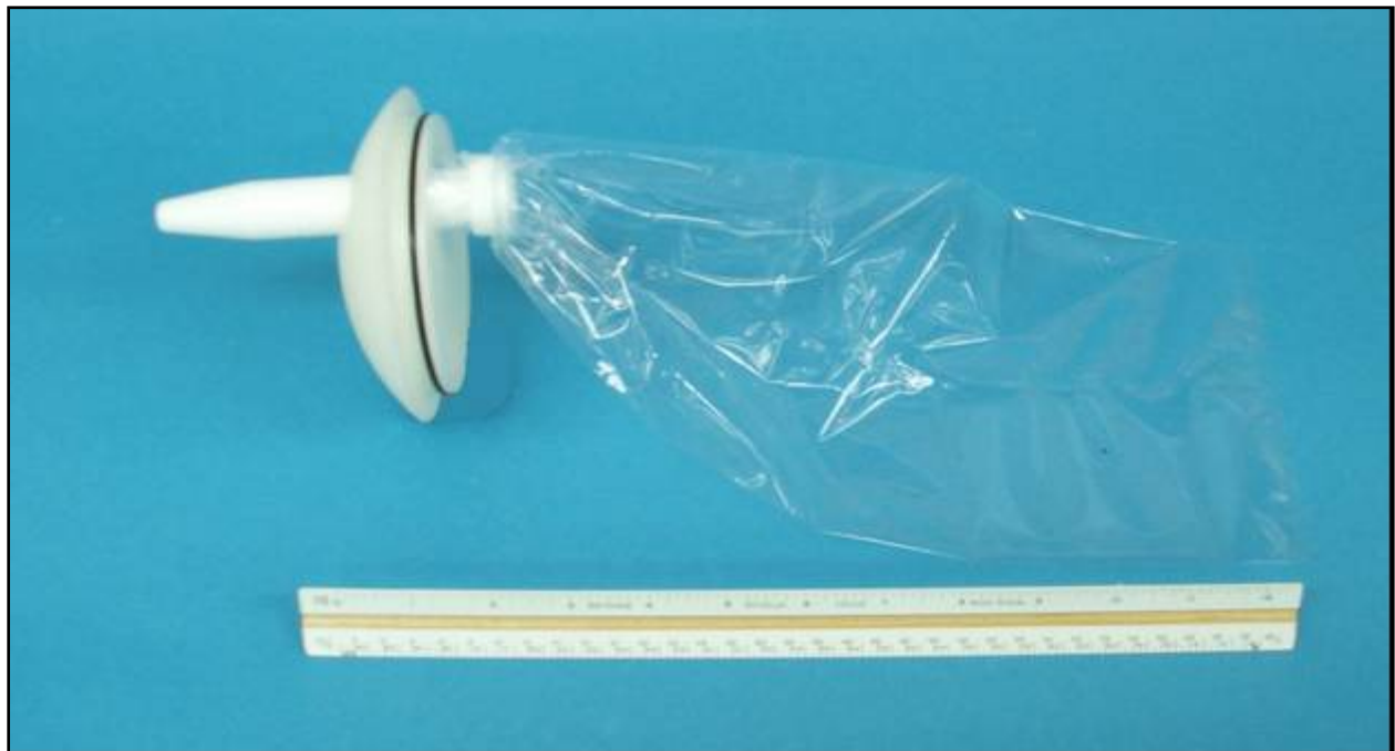
Figure 6 US DH-2 nose, nozzle, nozzle holder and bag assembly.
