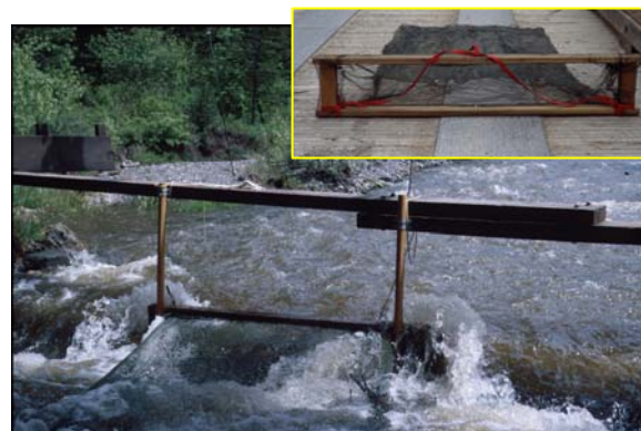
Figure 2: Net-frame sampler installed
