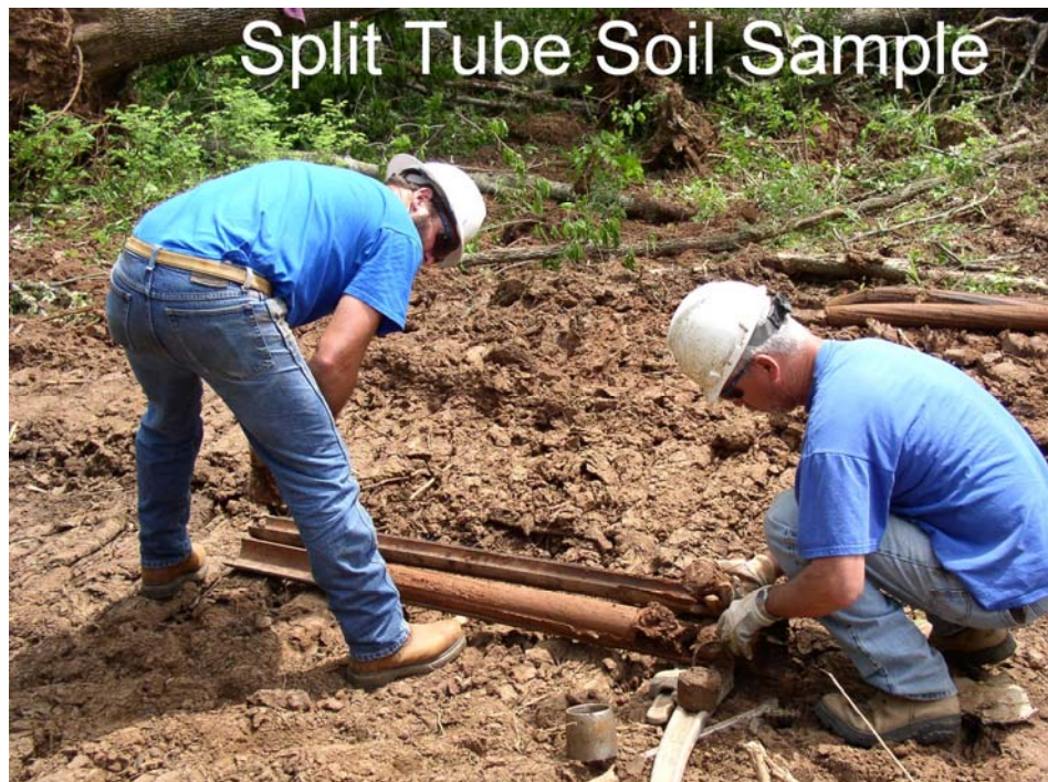
Figure 2 Collecting Split Tube Soil Samples, Oklahoma.
