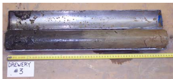
Figure 6 A picture of the vibracore sample at Drewery #3 after the aluminum casing has been split in half showing an interface at approximately 26 cm.
