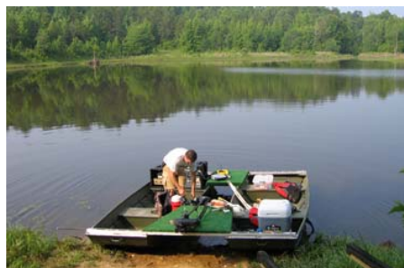
Figure 4 Pontoon style boat built by connecting two small Jon-boats together. This platform allows measurements to be taken in very shallow water.
