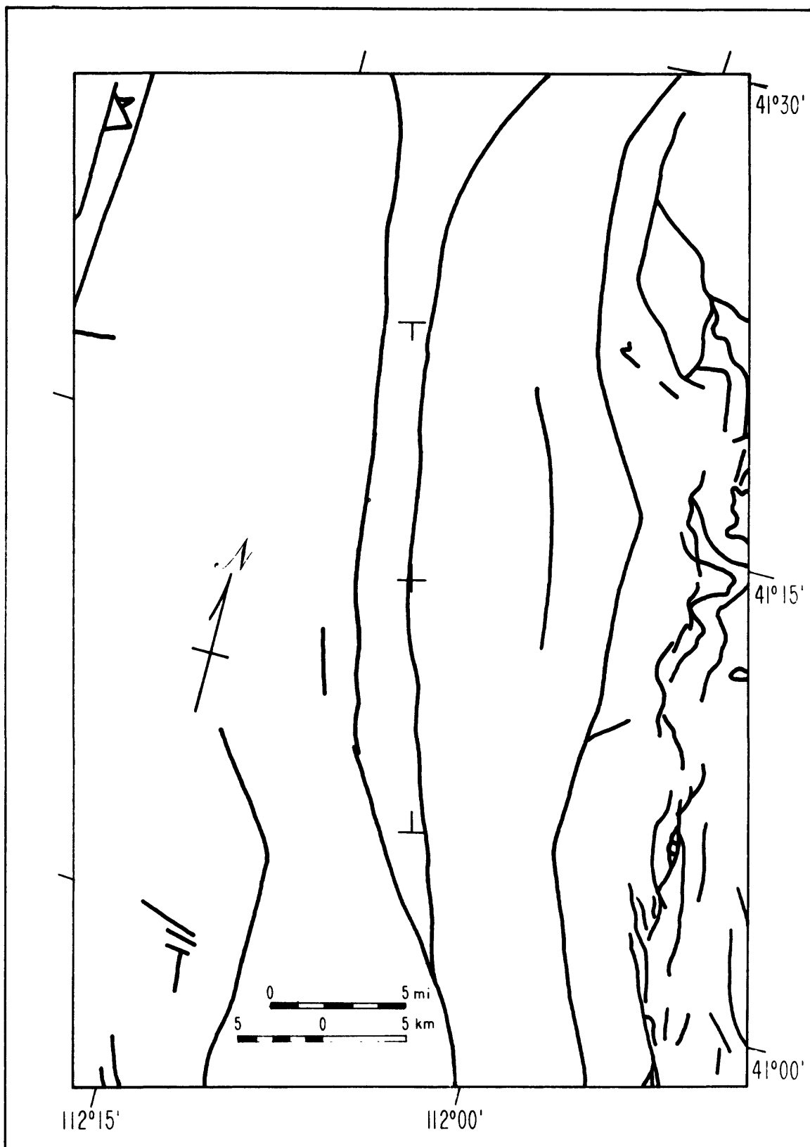
Figure 19.--Area of probable faulting for the Ogden distant event. + indicates the assumed epicenter; \perp and \top indicate the ends of the assumed fault.
