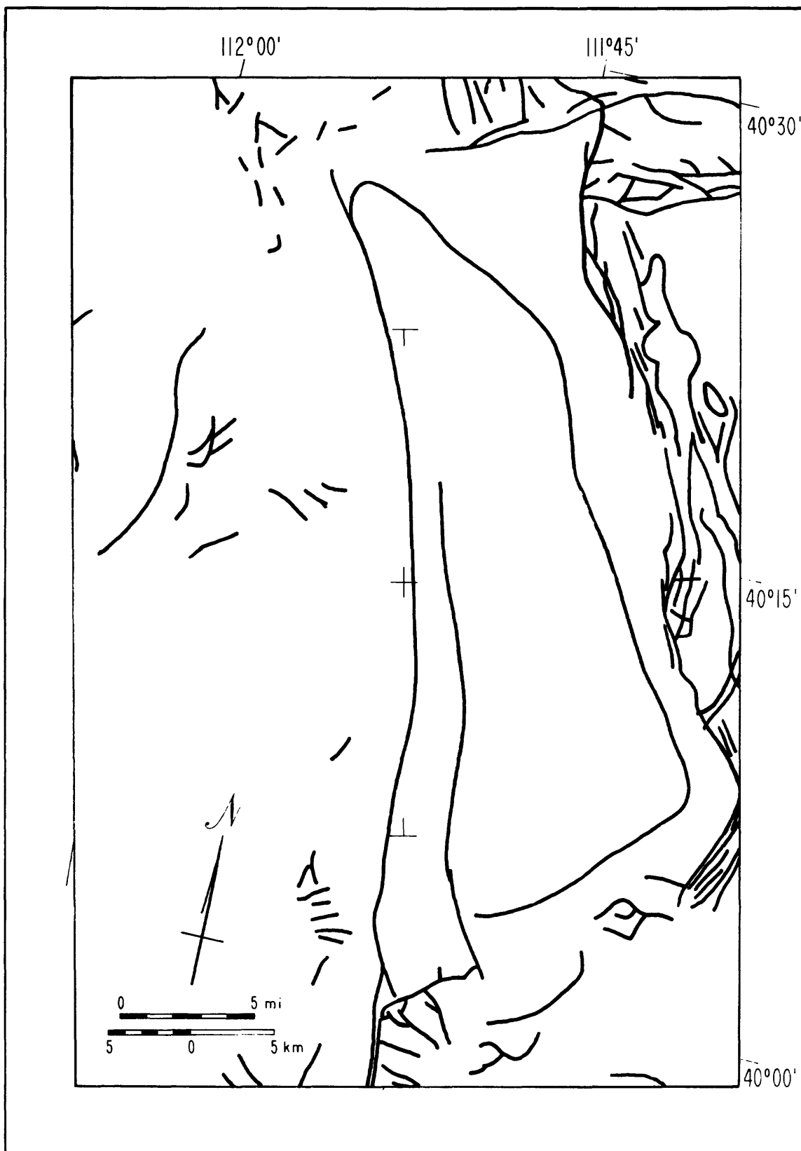
Figure 17.--Area of probable faulting for the Provo distant event. + indicates the assumed epicenter; └ and ┘ indicate the ends of the assumed fault.
