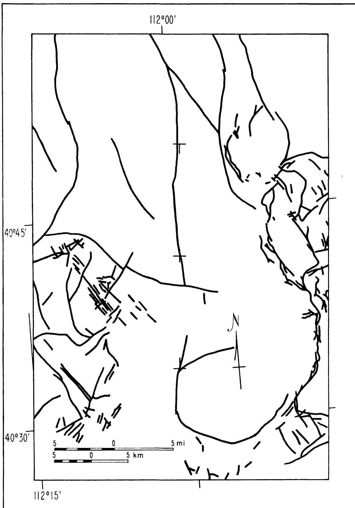
Figure 15.--Area of probable faulting for the Salt Lake City distant event. \times indicates the assumed epicenter; \perp and \top indicate the ends of the assumed fault.
