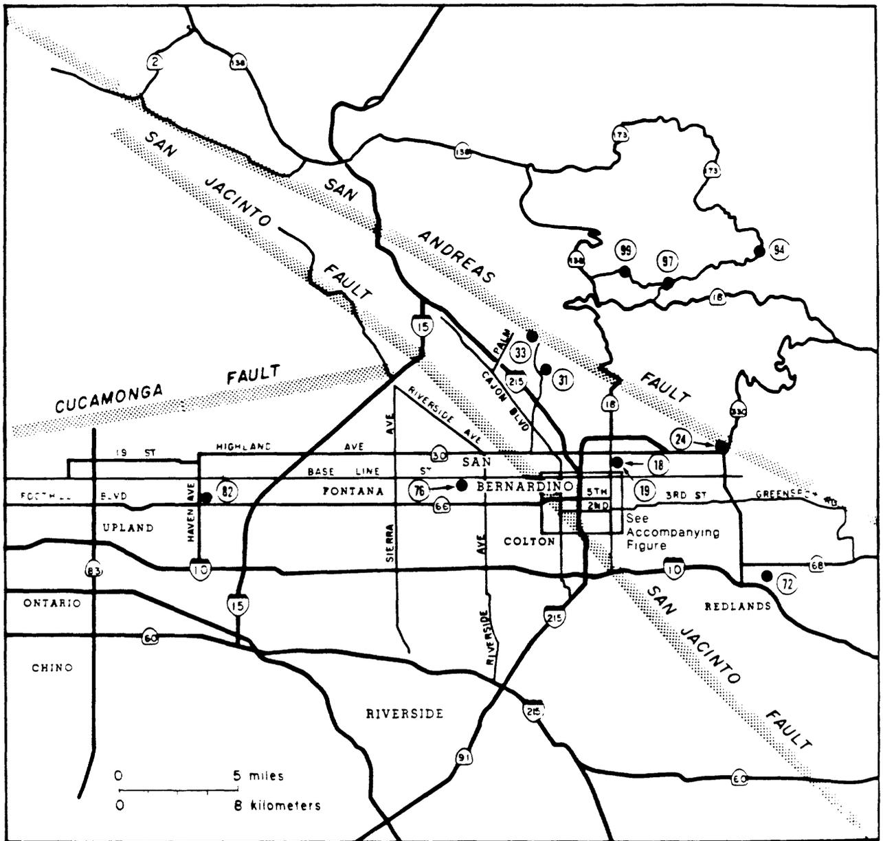
Figure 1. Locations of structures on final priority list for seismic instrumentation, San Bernardino County, California. The structures are identified by their numbers from Table. 2.
