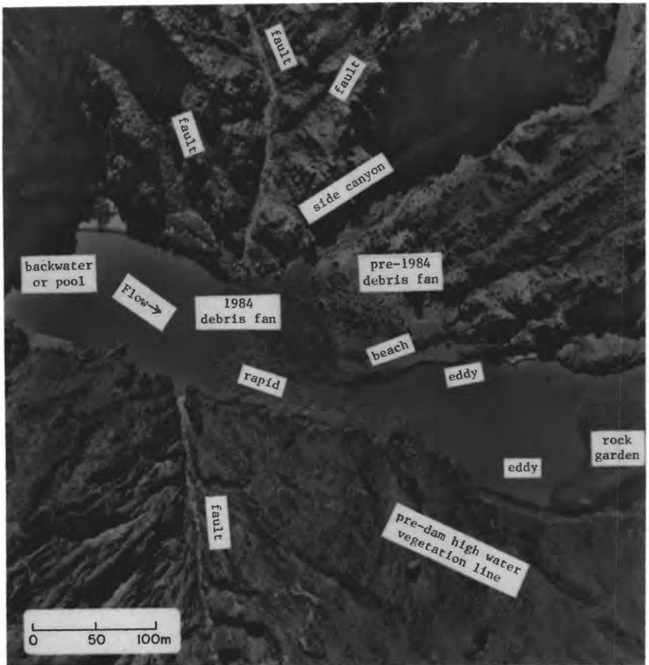
Figure 2. (a) Aerial photograph of Granite Rapids at a discharge of 5,000 cfs, showing the geomorphic features common to many rapids. For definitions of the terms, see text. Photograph by U.S. Bureau of Reclamation, 1984. Regional faults from Dolan, Howard and Trimble (1978). (b and c) Aerial photographs of Granite Rapids at 30,000 cfs showing typical wave structures in rapids. Photographs by U.S. National Park Service. (b) is at the same scale as (a); (c) is enlarged so that individual hydraulic features can be identified.
