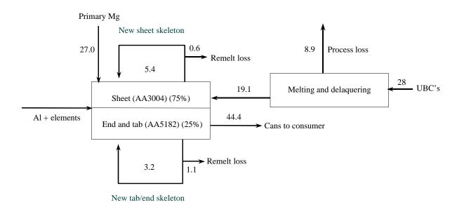
Figure 4. Simplified used beverage can processing, in thousand metric tons contained magnesium. UBC's, used beverage cans. (Adapted from Bowman, 1983.)
