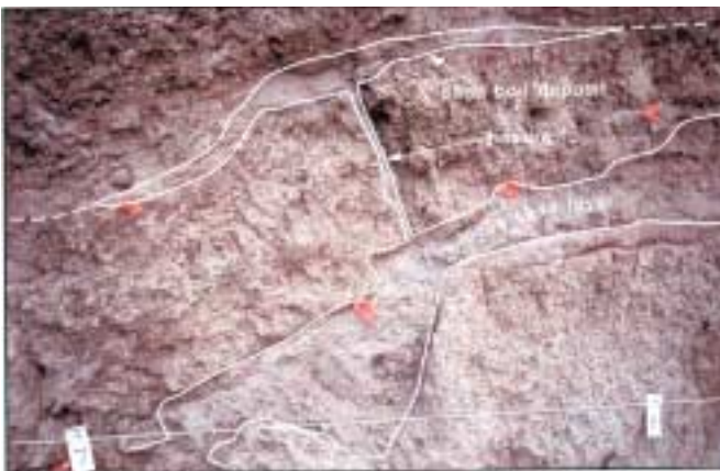
Figure O-4. Cross section of fossil sand boil in stream bank adjacent to Honey Lake fault zone. Loose sand that liquefied was forced through fissure in overlying soil and erupted onto ground surface. That surface was then rapidly buried by stream sediments, thereby preserving the sand boil. Sand boil deposit was tilted by deformation related to later earthquakes. White tags are 1 m apart. Photograph by C.J. Wills, 9/20/1990.
