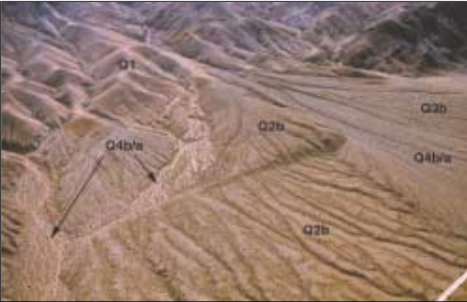
Figure A3-6. Offset of Q2b surface along Northern Death Valley fault near Anticline Ridge (see fig. A1-2). Note that Q2b deposits have a lighter tone due to carbonate rubble and retain alluvial fan morphology unlike deeply dissected older Q1 deposits that form ballenas near fan apex (photograph by J.R. Knott).
