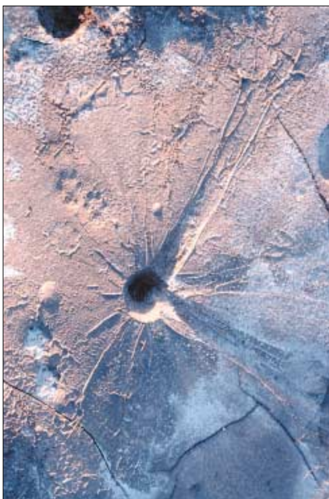
Figure O-1: High-angle oblique view of a sand boil at U.S. Geological Survey Wildlife Test Array in Imperial Valley, Calif. Superstition Hills earthquake of November 1987, caused liquefaction of fine sand from a layer about 2 m below surface. Sand erupted through a narrow fissure and flowed over surface, producing a sand boil. Note human and canine footprints for scale. Photograph taken by C.J. Wills, 2/8/1988 from about 1.5 m above surface.
