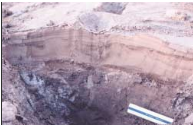
Figure O-2. Cross section of sand boil in Imperial Valley. Superstition Hills earthquake of November 1987 caused liquefaction of fine sand from a layer about 2 m. below the surface. Liquefied sand erupted through a narrow fissure and flowed over the surface. Surface crater is approximately 10 cm (4 inches) in diameter; Holzer and others (1989) described this site in detail. Photograph by C.J. Wills, 2/8/1988.
