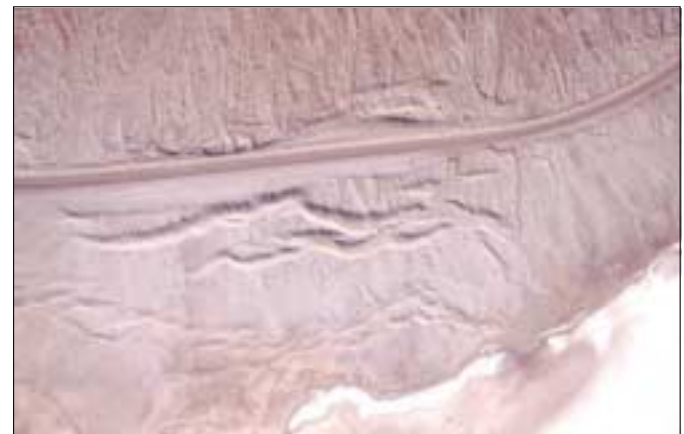
Figure O-6. Near vertical view of lateral spread at toe of the Bad Canyon alluvial fan, 0.4 km SW of Badwater. Note well-developed graben in center of area, sharper and somewhat arcuate scarps around upslope margin of feature above (south of) the road and smaller ridges at edge of playa, possibly representing compressional deformation. Highway indicates scale. Photograph taken from about 300 m (1,000 ft) altitude by M.N. Machette, Nov. 2000.
