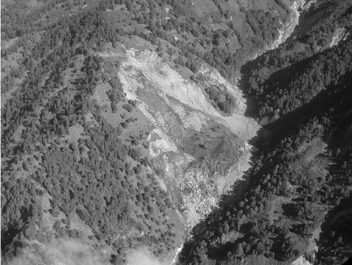
Figure 4. Oblique aerial view to north of the landslide that produced the dam on the Río La Lima, photograph by Jeffrey Coe taken 12 January 2001. Smooth even-toned surface crossed by Río La Lima at the toe of the landslide is the sediment fill behind the landslide dam.
