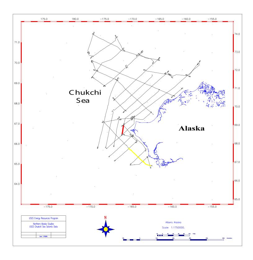
Figure 1. - Tracklines of the Chukchi Sea seismic survey. Highlighed in red is the line shown in figures 2-3. Highlighted in yellow is the unrecoverable segment of line 19.
