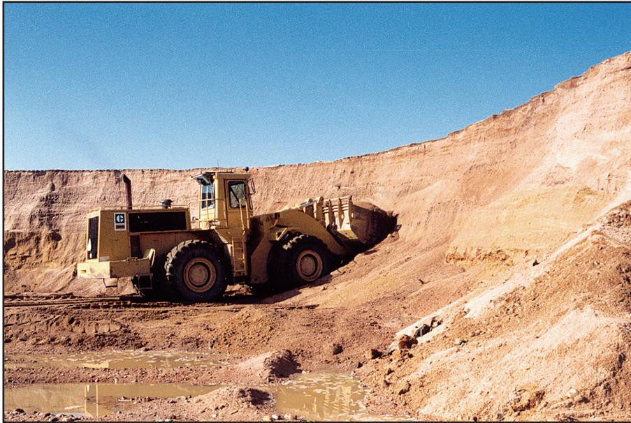
**Figure 11.** If sand and gravel is above the water table it can be excavated using conventional equipment. (Photo by W.H. Langer, USGS)
