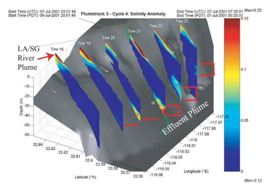
**Figure 10-6**. Cross-shelf section of salinity anomaly from cruise 3, cycle 4, a period of weak flow over the continental shelf off Huntington Beach. The salinity anomaly indicates that the plume is present in both alongshore directions extending away from the outfall diffuser at a depth of between 25 and 50 m. The salinity anomaly also shows the presence of the Los Angeles/San Gabriel River plume nearshore at the surface.
