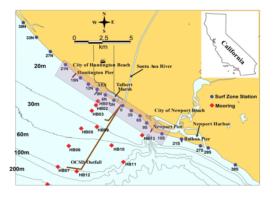
**Figure 2-3.** Map of the coastal zone surrounding Huntington Beach, California. The blue dots show the location of the surfzone sampling stations from 39N to 39S. The outfall is shown leaving the coast near station 0. The diffuser of the outfall is located near stations HB07 and HB12. Station 12S is located at Newport Pier.
