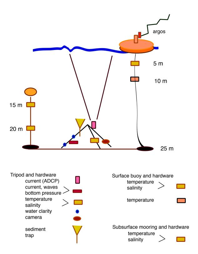
Figure 2-7d. Schematic of moorings at site HB05.
