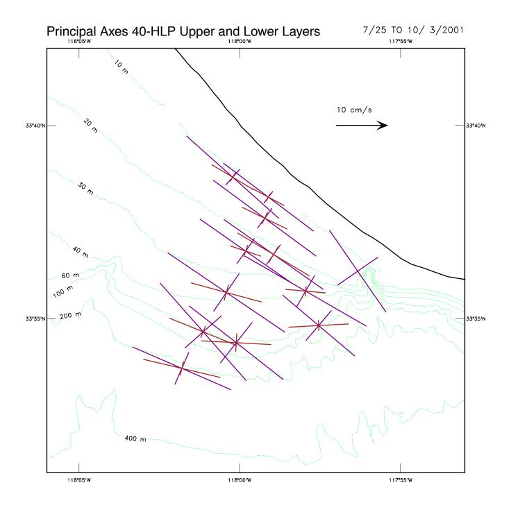
**Figure 4-7.** Principal axis directions from 40-HLP velocity data for the upper (purple) and lower (brown) layers. The lower-layer instrument depths are the same as in Figure 4-6.
