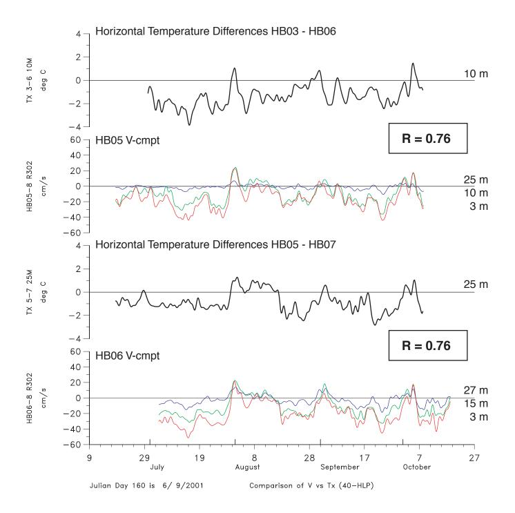
**Figure 4-8.** Comparison of the along-isobath component (V) of 40-HLP currents with horizontal temperature differences between moorings onshore and offshore of the current measurements on the middle shelf. Correlation coefficient, R, is between the temperature differences and the 3-m velocity component.
