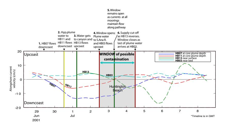
**Figure 5-2.** Alongshore current velocity curves for a hypothetical contamination event from the Newport Canyon pathway showing the six conditions to define an event. Solid sections of colored lines show the velocities and mooring used per leg of transport to determine whether hypothetical plume water reached Huntington Beach to intially open the window.
