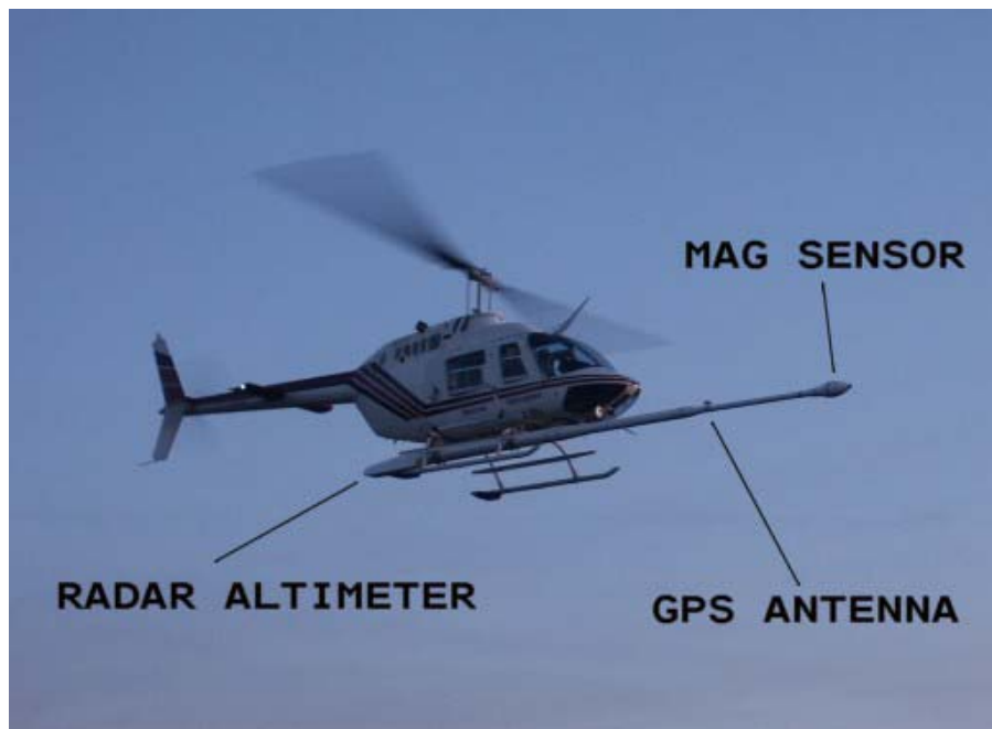
Figure 4: HM1 platform system
