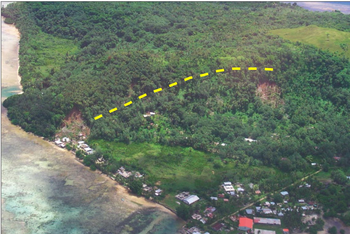
Figure 15. Oblique aerial view of Sapore slump/debris flow (left center) on the island of Fefan. Dashed line indicates approximate position of reactivated head scarp of preexisting large incipient slump. Preexisting slump mass is below and to the right of dashed line.
