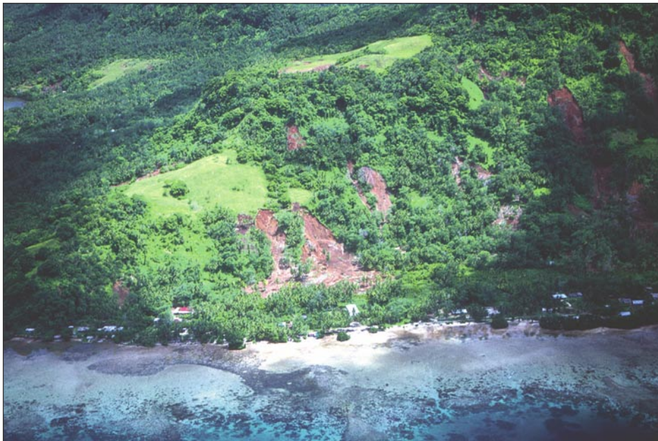
Figure 13. Aerial view of Pwene slump/debris flow on the island of Fefan. This site shows a debris-flow doublet (center of photo) with a downslope line of trees located on a ridge between the two debris flows that coalesced.
