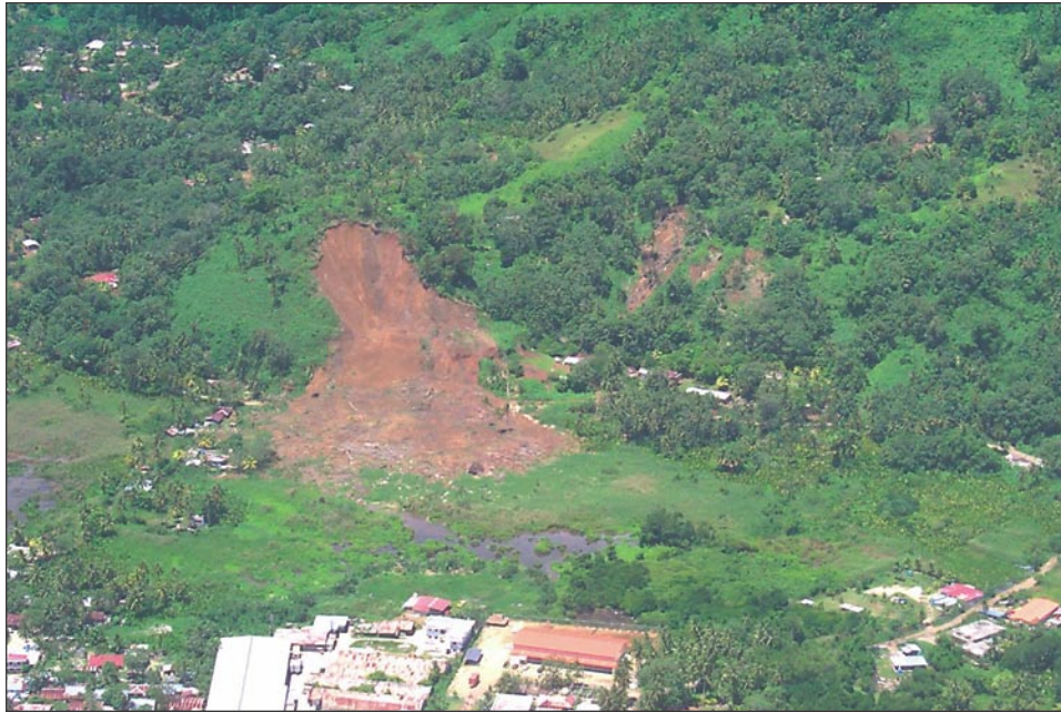
Figure 6. Oblique aerial photograph of Nepukos slump/debris flow on the island of Weno.
