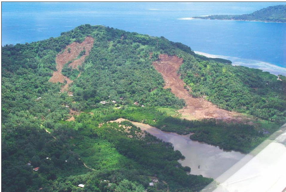
Figure 10. Oblique aerial view of Kuchua slump/debris flow (right) and Roro debris slide/flow (left) on the island of Tonoas.
