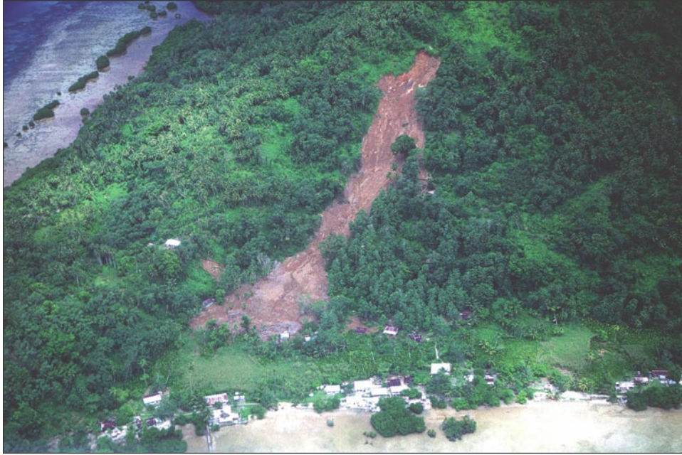
Figure 19. Aerial oblique view of slump/debris flow at the village of Penia on the island of Udot.
