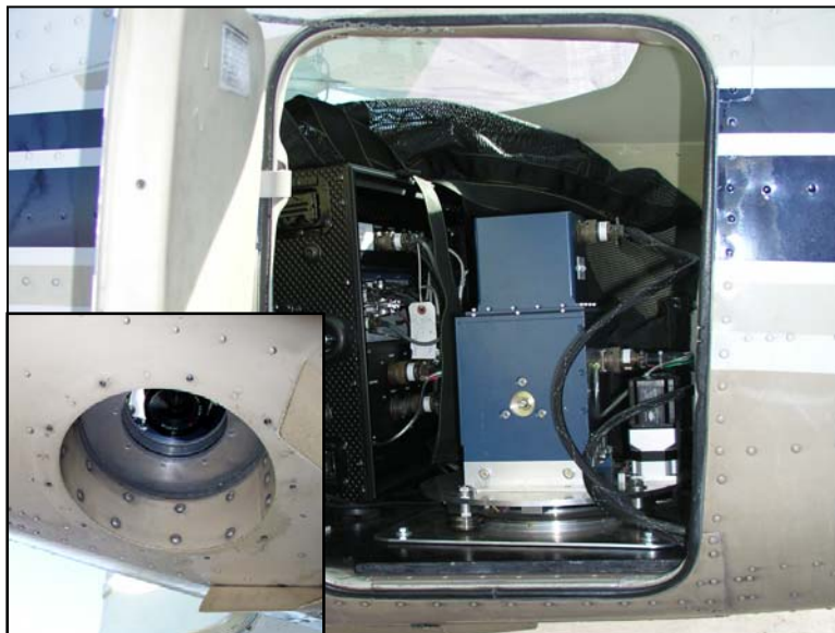
Figure 2. View of mounted DSS and inset of camera port hole under the aircraft.
