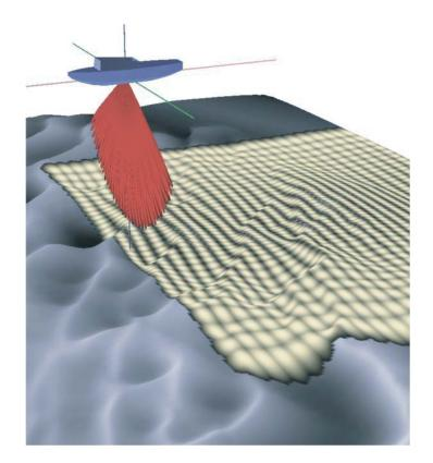
**Figure 2.1.** Schematic showing the operation of a multibeam sea floor mapping system. In water depths ranging between 5 and 200 m, the EM1000 mapping system generates an aimed array of 60 beams, spaced at intervals of 2.5 degrees, that insonify a strip of sea floor measuring in width approximately 7.5 times the water depth. In the Massachusetts Bay survey, the horizontal spatial resolution of the data is 5-10 m and the vertical resolution is approximately 50 cm.
