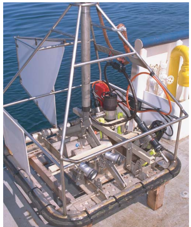
Figure 2.3. The USGS SeaBed Observation and Sampling System (SEABOSS) used to obtain still photographs, videos and obtain samples of the sea floor sediments. These observations are used to help interpret the backscatter intensity obtained in the multibeam surveys. The SEABOSS is lowered to within about a meter of the sea floor and obtains photographs and videos as the ship drifts over selected features. A single sample of the bottom sediments may be obtained during the photographic transect. Top: A view of the SEABOSS from below (with base plates removed). The instruments are as labeled: A, forward-looking video camera; B, lights for forward-looking video camera; C, downward-looking video camera; D, lights for downward-looking video camera; E, 35-millimeter still camera; F, strobe light for still camera; G, modified Van Veen grab sampler; H, depth sensor; I, junction box; J, parallel lasers for scale; K, angled laser for range. Right: SEABOSS on deck.
