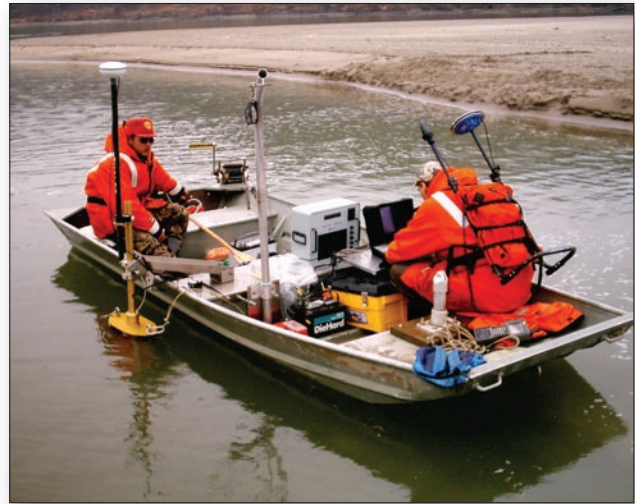
Figure 4. Configuration of instruments used in bathymetric and water-velocity data collection.
